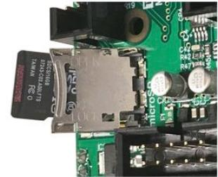
1: The SD card is mounted to the back of the Tête in a small metal door.
