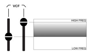
Lowering the **LOWPASS FREQ [30]** slider removes high frequency content from the signal. As a result, the position of both sliders gives a visual representation of the frequency band passing through the filter.
