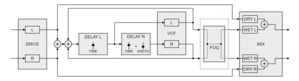
If ALT FB CROSS [8] is enabled, then crossing the feedback reverses the order of the delays, with the left delay following the right in the serial chain:
