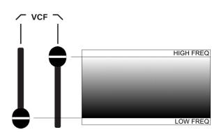
Raising the **HIGHPASS FREQ [28]** slider removes low frequency content from the signal.
