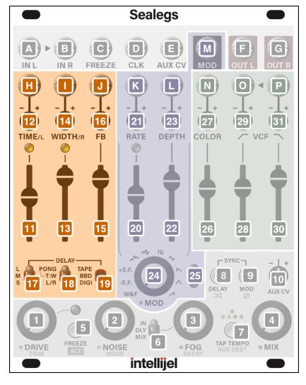
When un-sync'd, and free-running, the slider works over a range of 3.125 ms - 93.75 ms; 50 ms - 1.5 s; or 200 ms - 6 s, as set with the **TIME RANGE** [17] switch.
