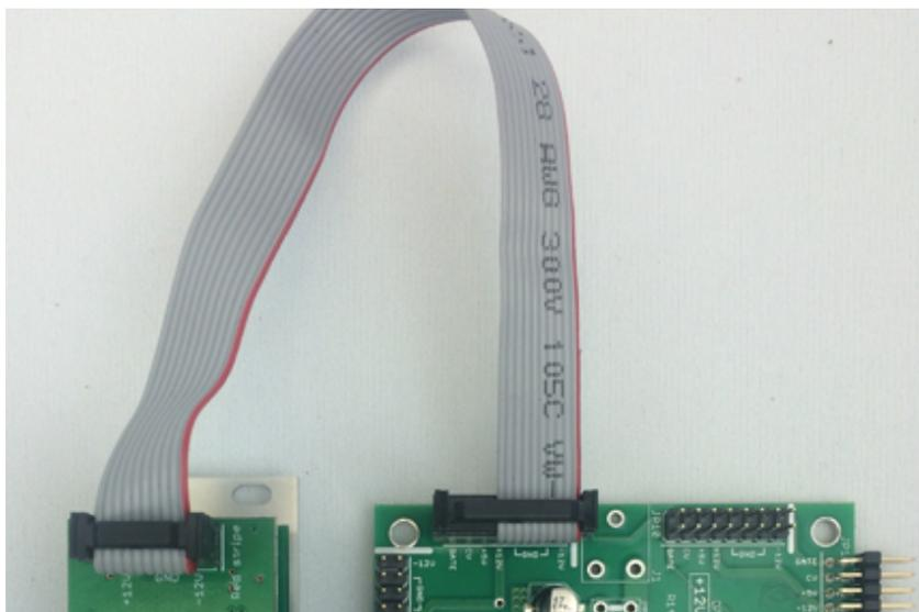
Before reconnecting power and turning on your modular system, double check that the ribbon cable is fully seated on both ends and that all the pins are correctly aligned. If the pins are misaligned in any direction or the ribbon is backwards you can cause damage to your module, power supply, or other modules.
