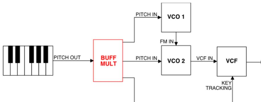
Unlike a passive mult, which merely splits the incoming signal and shares it across multiple outputs (much like a Y-cable), buffered mults make electrical copies of an input voltage and duplicate that voltage at the outputs.
