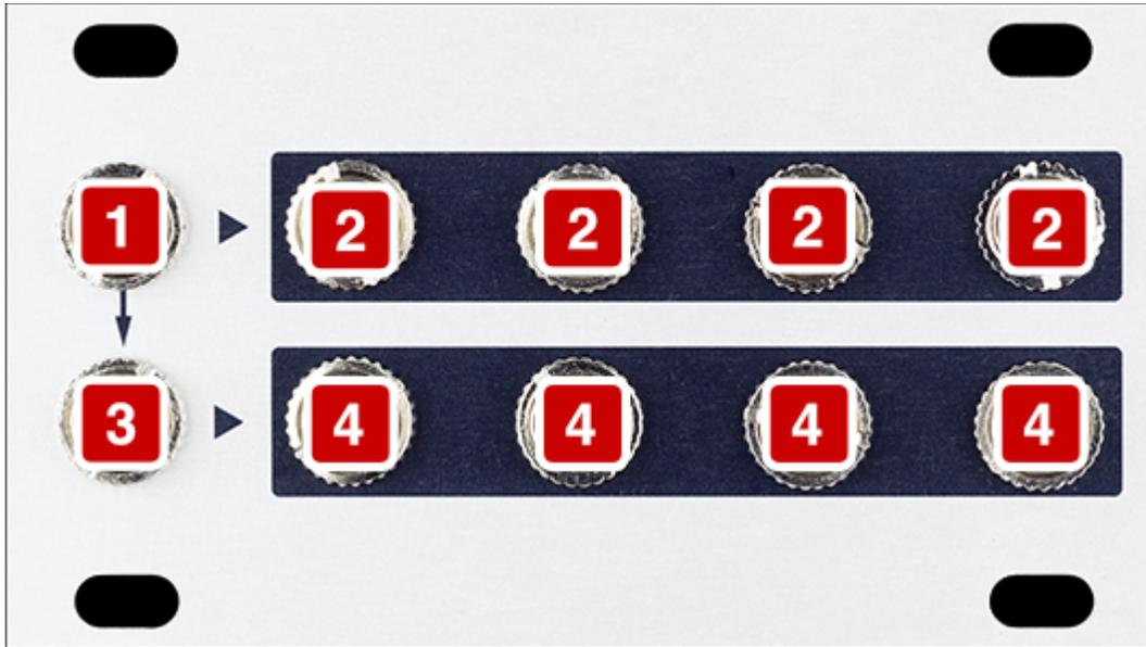
Buff Mult 1U is a dual 1 x 4 buffered signal multiplier. A signal multiplier takes an input signal and routes it to multiple outputs simultaneously. For example, you might want to route keyboard's pitch CV to three different destinations: one to govern the pitch of your main oscillator; another to govern the pitch of a second oscillator; and the third to open and close a filter so that it tracks across the keyboard.
